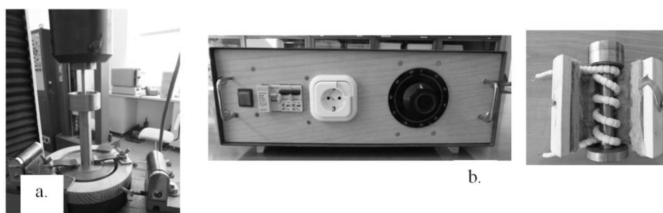
Fig. 2. Punch and the temperature control and measurement system
